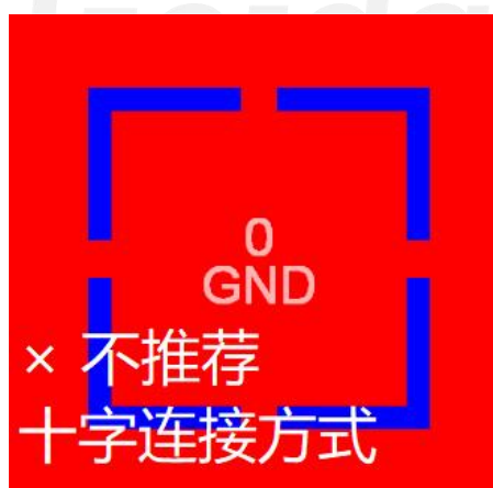
Figure 5.4 Unrecommended Copper Laying Connection
