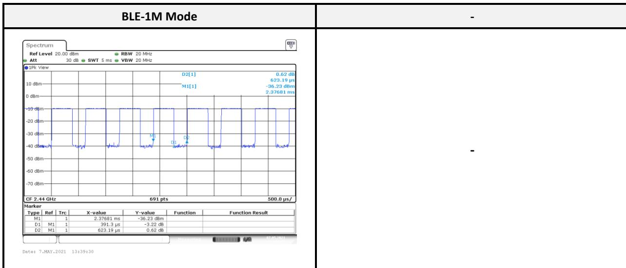
\*Note: Duty Factor =  $10 \times \log(1/\text{Duty cycle})$
