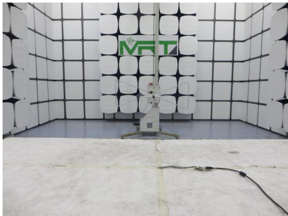
Description: Radiated Emission Test Setup Photos above 1GHz
