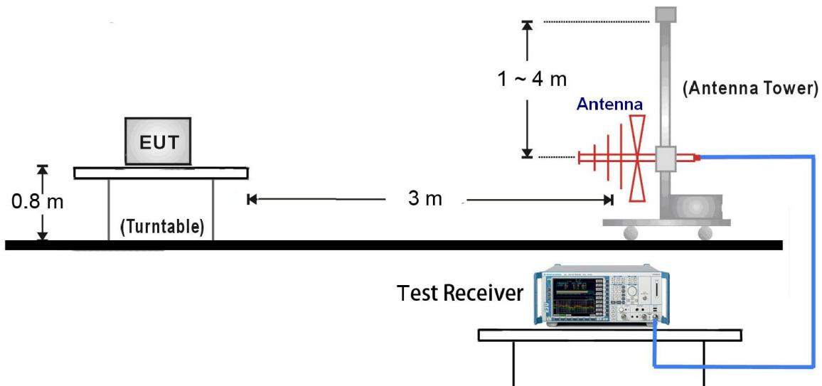
1GHz ~ 18GHz Test Setup:
