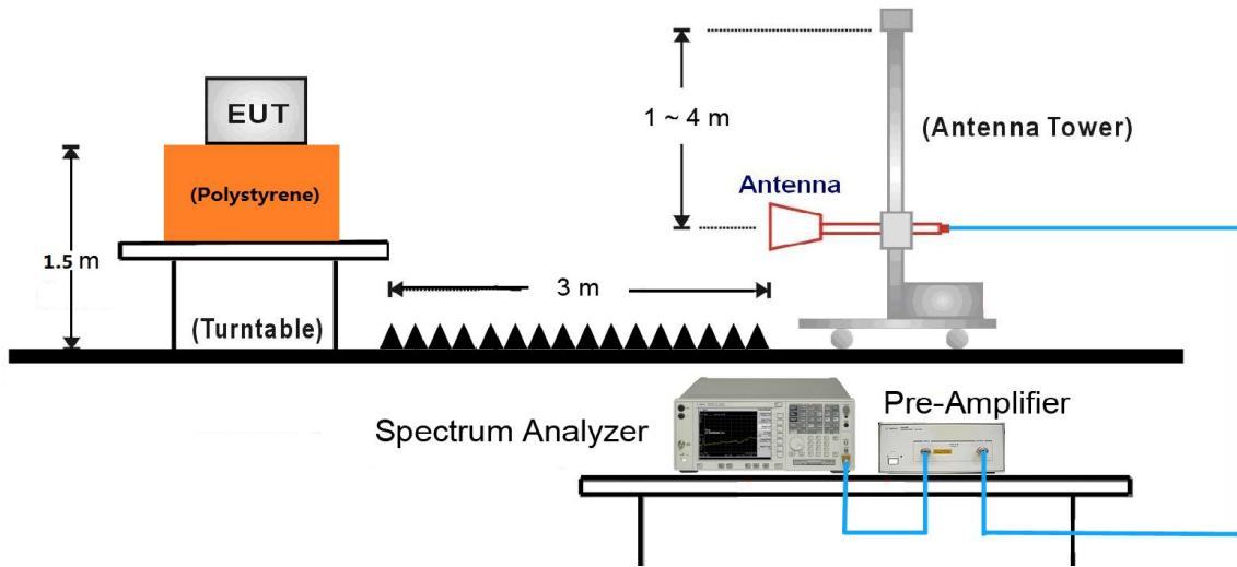
18GHz ~25GHz Test Setup:
