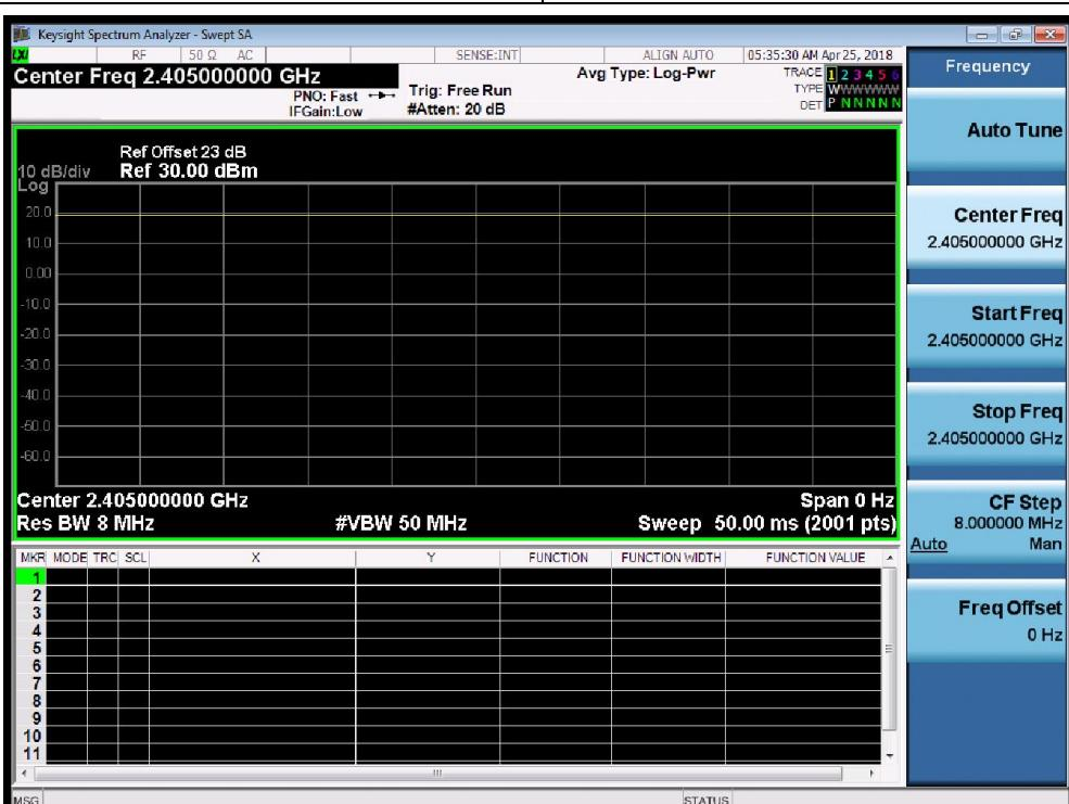
The screenshot shows the Keysight Spectrum Analyzer software interface. The main display shows a signal at 2.405 GHz with a 50 MHz VBW and 8 MHz Res BW. The right side of the screen displays a control panel with the following settings:
