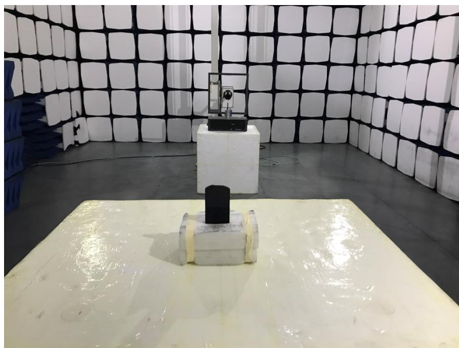
**Radiation Emission Test Setup (30MHz to 1GHz)**
