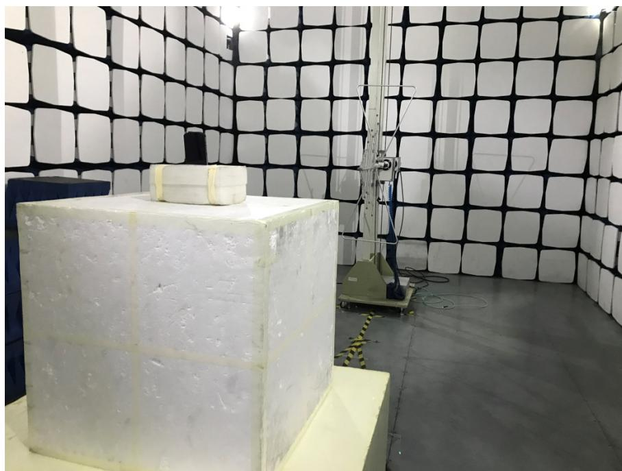
**Spurious Radiation Test Setup (1GHz to 18GHz)**
