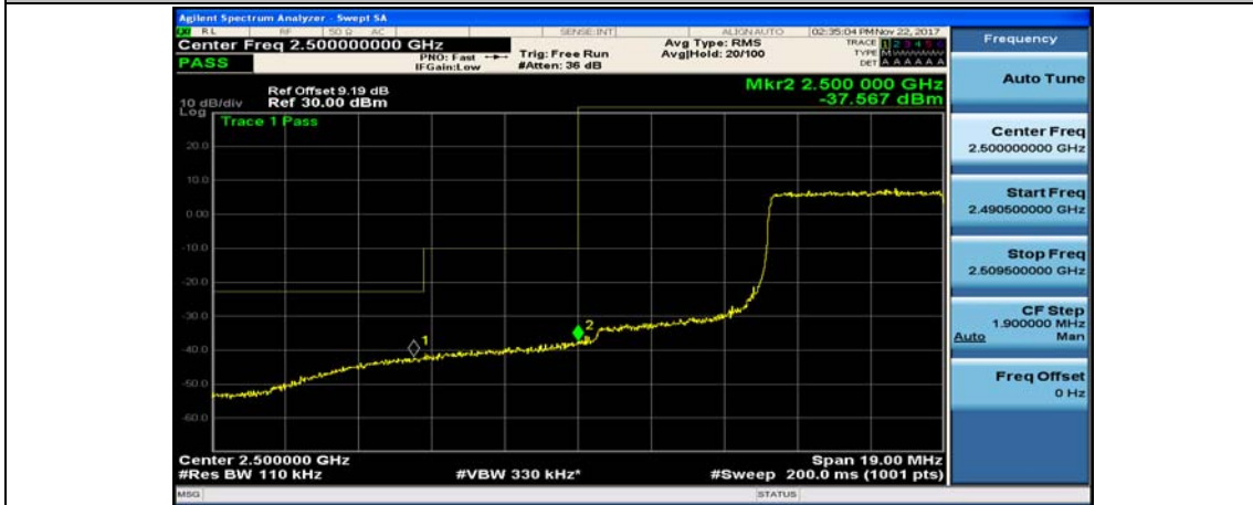
Channel Bandwidth: 10 MHz_LCH_16QAM_50RB#0
