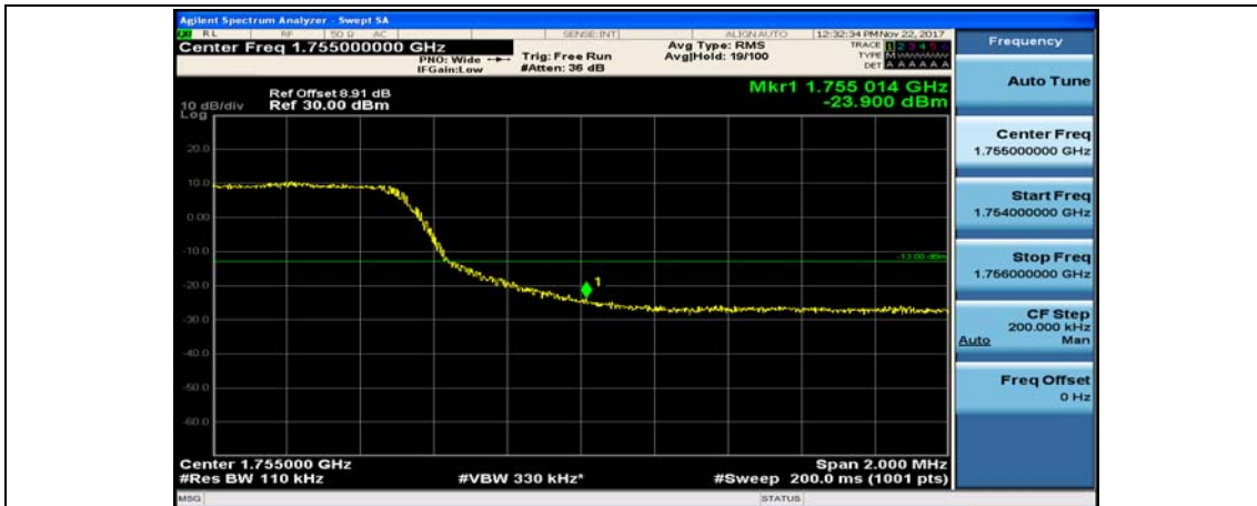
Channel Bandwidth: 10 MHz_HCH_QPSK_50RB#0
