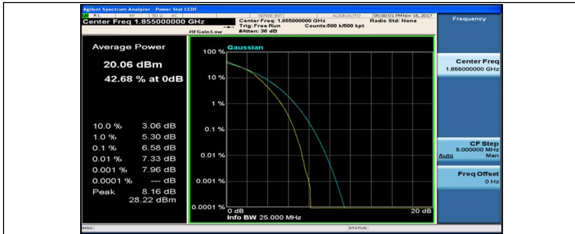
Channel Bandwidth: 10 MHz_MCH_16QAM_1RB#0
