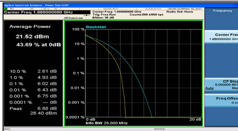
(Channel Bandwidth:15 MHz)_MCH_QPSK_75RB#0
