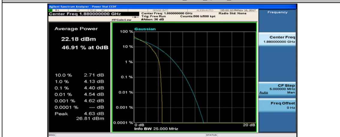
Channel Bandwidth: 10 MHz_MCH_QPSK_1RB#24
