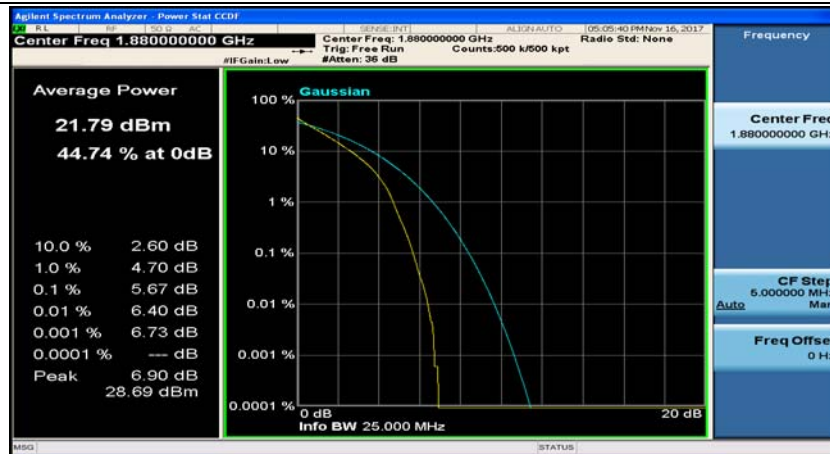
(Channel Bandwidth:15 MHz)_MCH_QPSK_75RB#0
