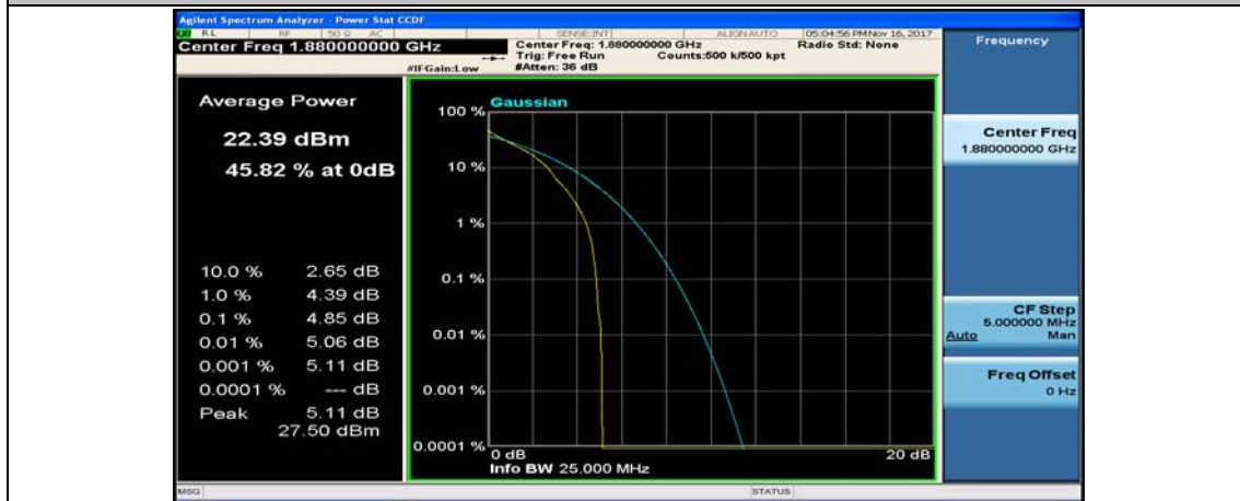
(Channel Bandwidth:15 MHz)_MCH_QPSK_1RB#74
