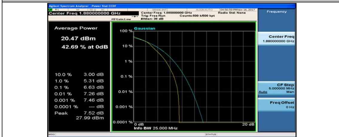
(Channel Bandwidth: 5 MHz)_MCH_16QAM_25RB#0
