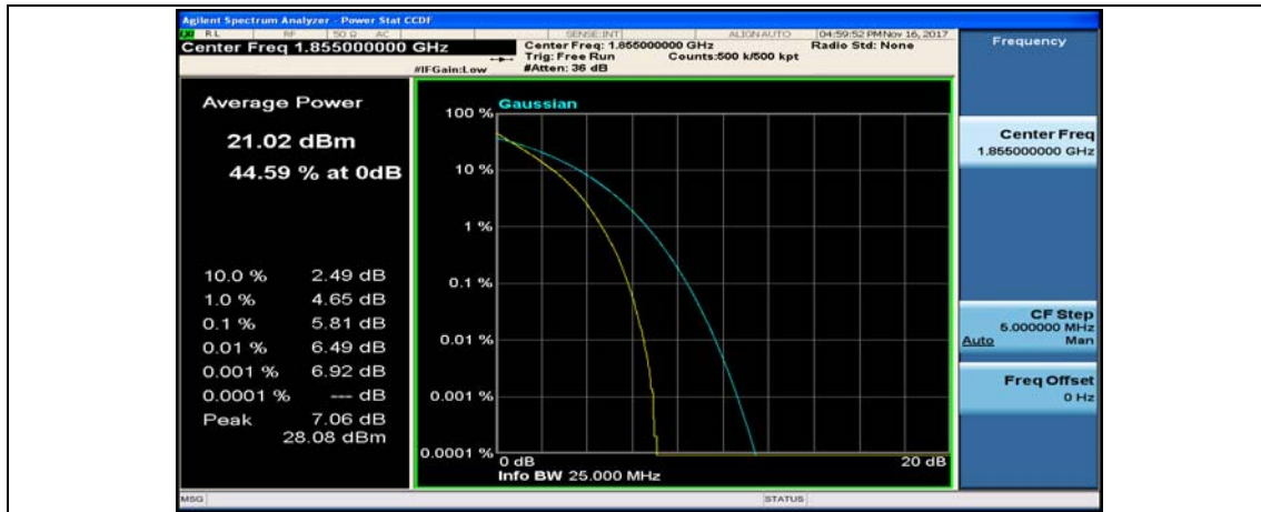
Channel Bandwidth: 10 MHz_MCH_QPSK_1RB#0
