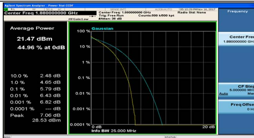
(Channel Bandwidth:20 MHz)_MCH_QPSK_50RB#50
