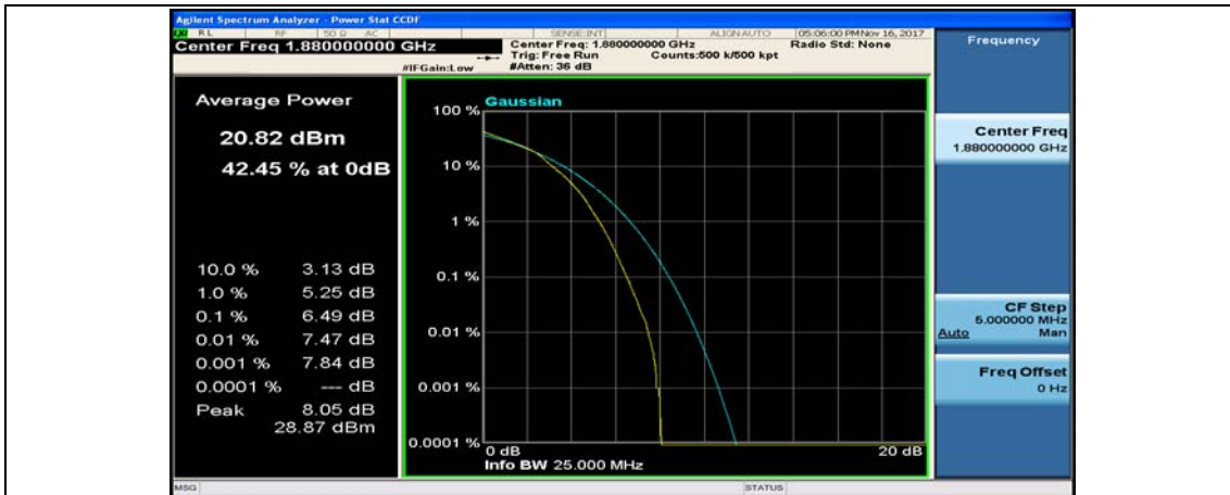
(Channel Bandwidth:15 MHz)_MCH_16QAM_75RB#0
