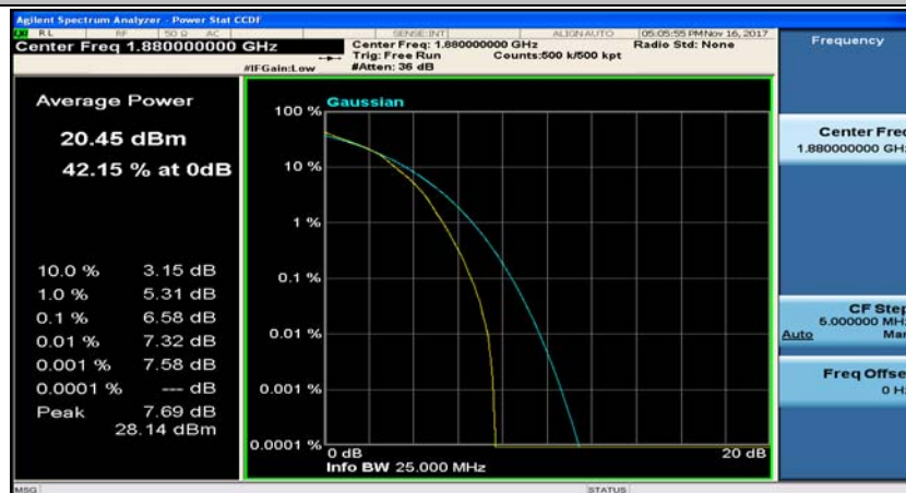
(Channel Bandwidth:15 MHz)_MCH_16QAM_37RB#38
