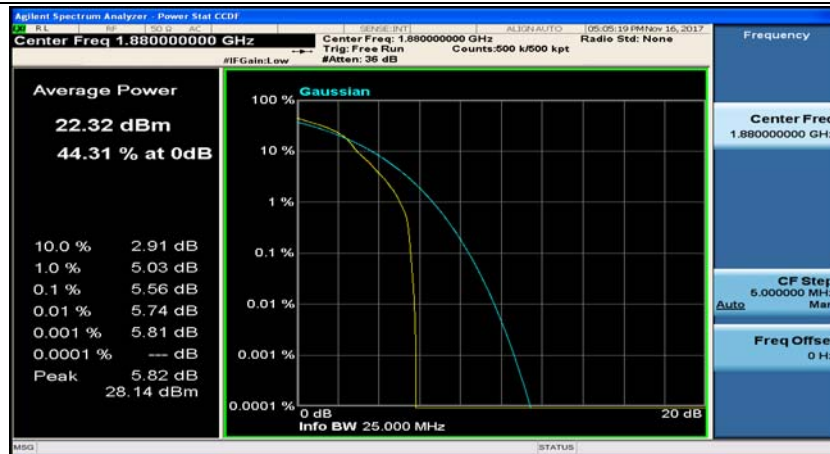
(Channel Bandwidth:15 MHz)_MCH_16QAM_37RB#0
