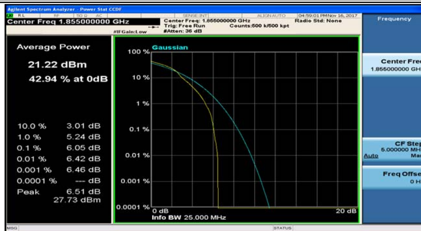
Channel Bandwidth: 10 MHz_LCH_16QAM_1RB#49
