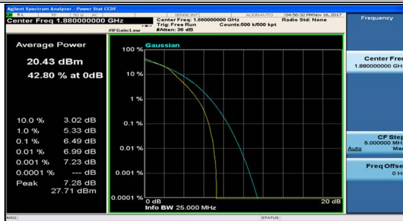
(Channel Bandwidth: 5 MHz)_MCH_16QAM_12RB#6
