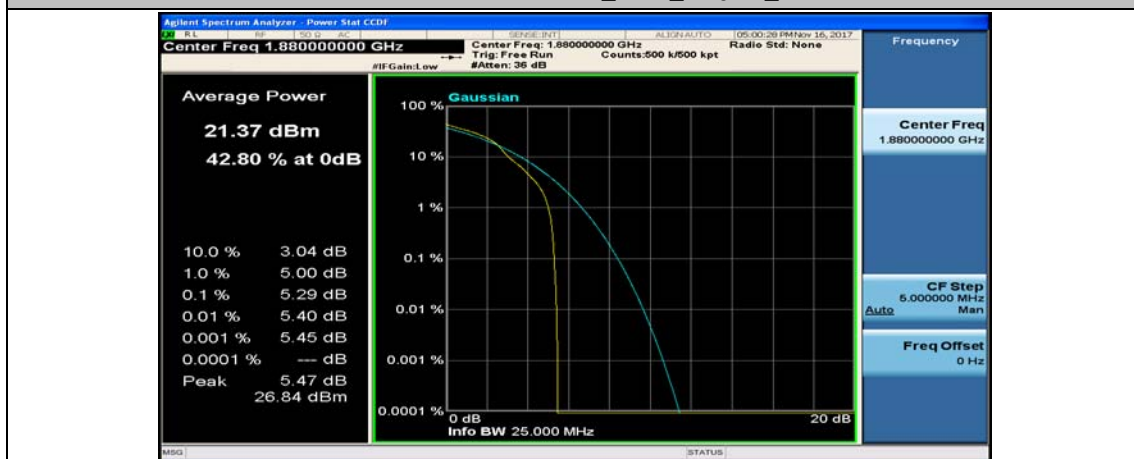
Channel Bandwidth: 10 MHz_MCH_16QAM_1RB#24
