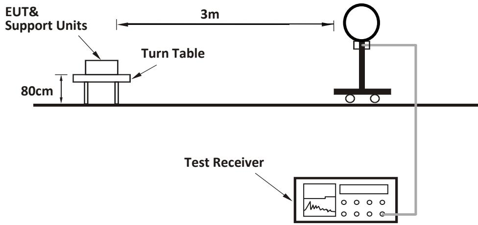
For Radiated emission 30MHz to 1GHz:
