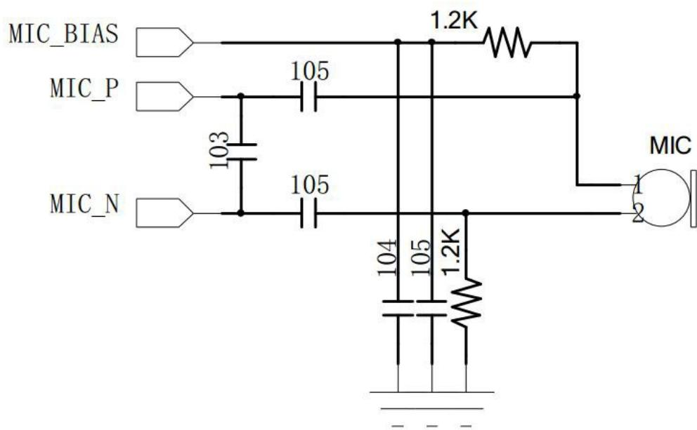
MIC recommended specification: sensitivity -38dB +/-2dB, working voltage: DC2V
