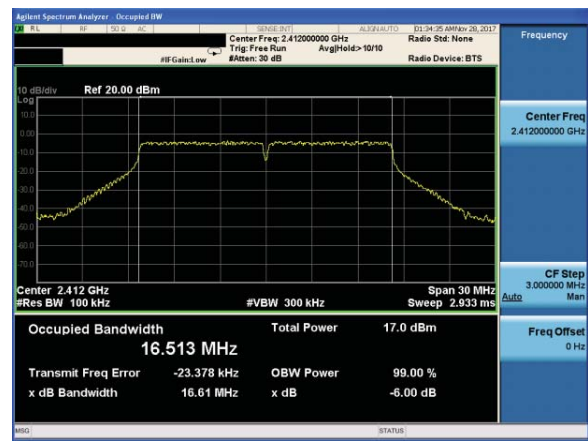
(802.11g) 6dB Bandwidth plot on channel 6
