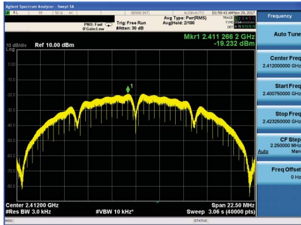
(802.11b) PSD plot on channel 6
