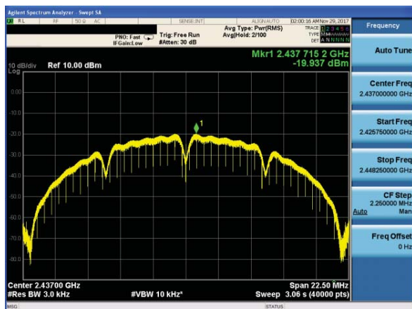
(802.11b) PSD plot on channel 6
