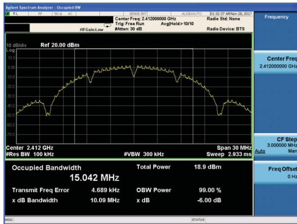
(802.11b) 6dB Bandwidth plot on channel 6
