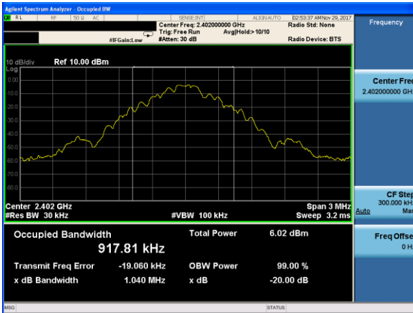
20dB Bandwidth plot on channel 39 (1Mbps)
