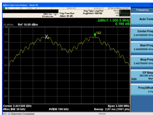
(1Mbps) Channel Separation plot on channel 39-40
