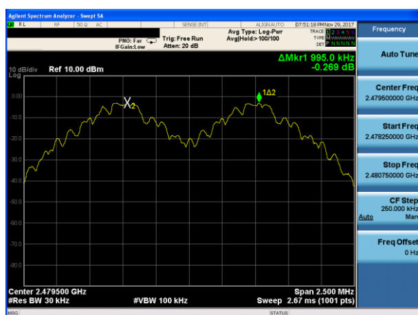
(1Mbps) Channel Separation plot on channel 77-78
