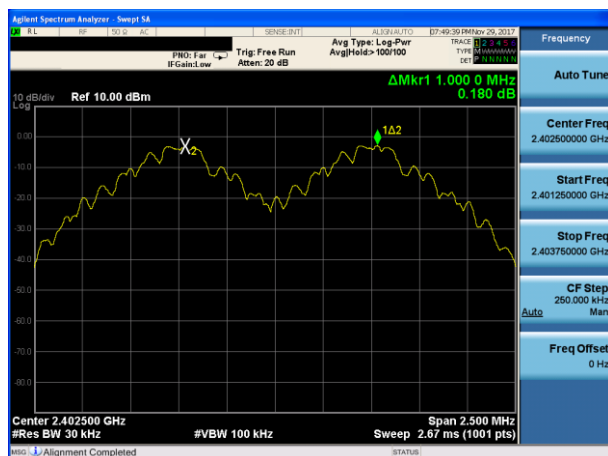
(1Mbps) Channel Separation plot on channel 00-01
