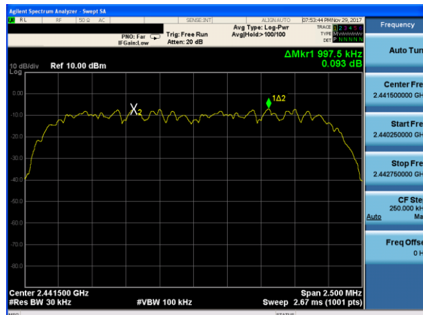
(2Mbps) Channel Separation plot on channel 39-40
