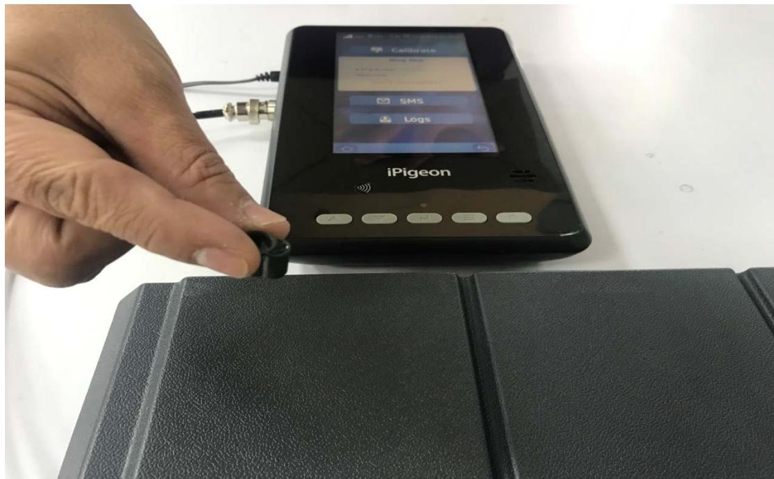
Place the electronic chip ring on the four-channel board (maximum above 5 cm) , each cell can be sensed
