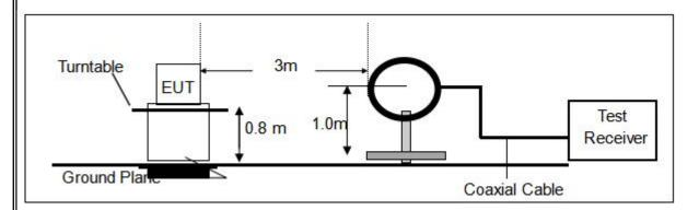
b) For Radiated Emission 30~1000MHz
