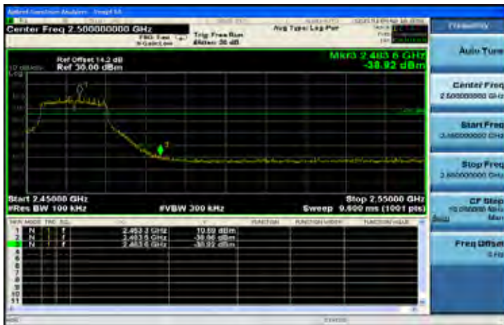
802.11g: Band Edges Test Data CH-High
