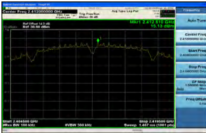
802.11b Reference Level of Emission Limit (CH-High)
