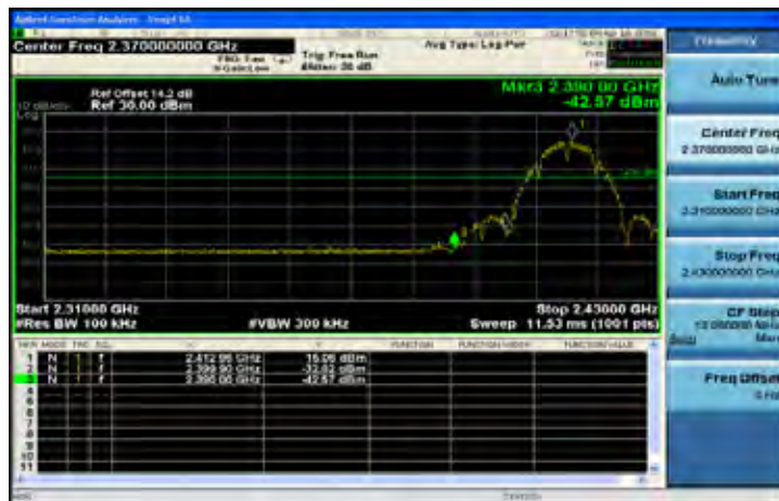
802.11b: Band Edges Test Data CH-High
