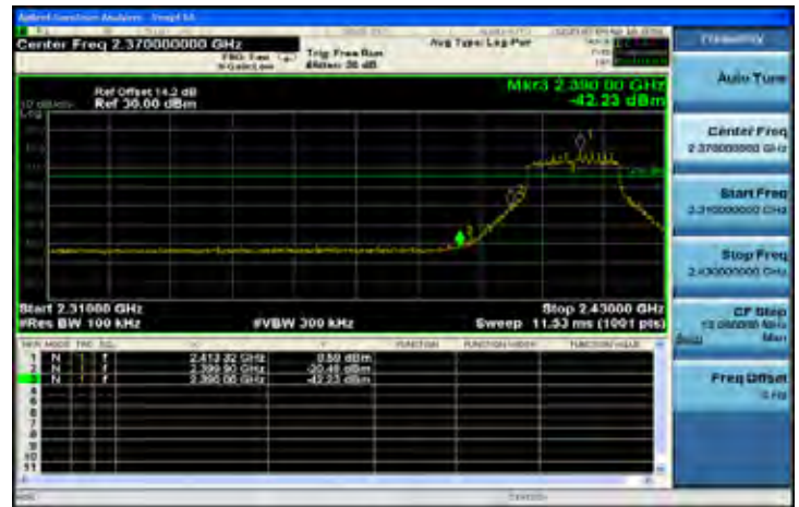
802.11n_HT20: Band Edges Test Data CH-High
