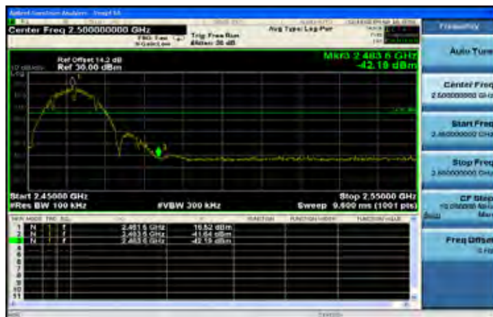
802.11b: Band Edges Test Data CH-High
