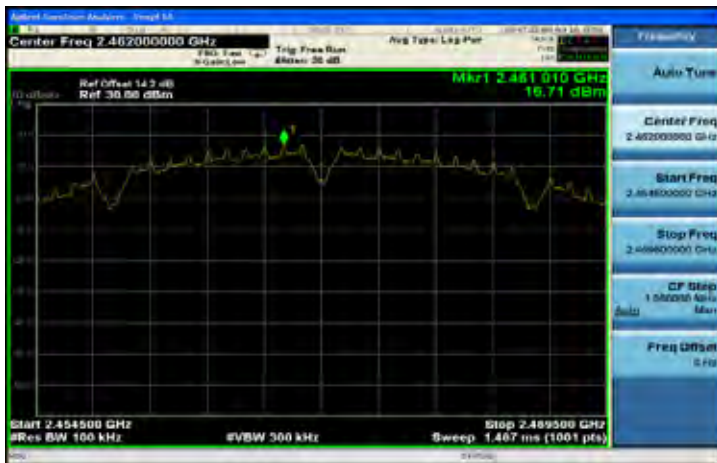
802.11b Reference Level of Emission Limit (CH-High)
