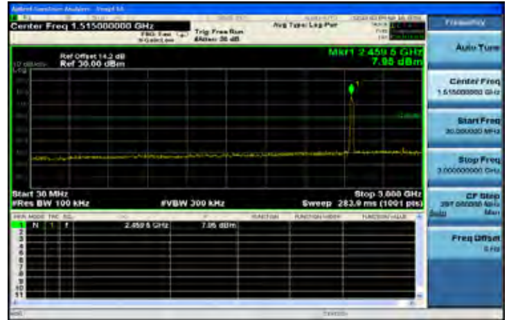
802.11g: Spurious Emission Test Data CH-High
