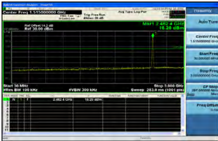
802.11b: Spurious Emission Test Data CH-High
