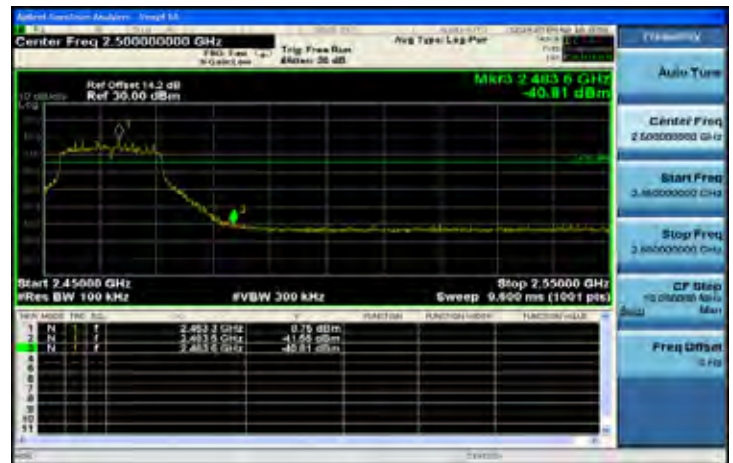
802.11n_HT20: Band Edges Test Data CH-High
