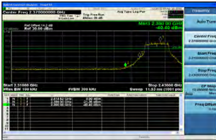
802.11g: Band Edges Test Data CH-High
