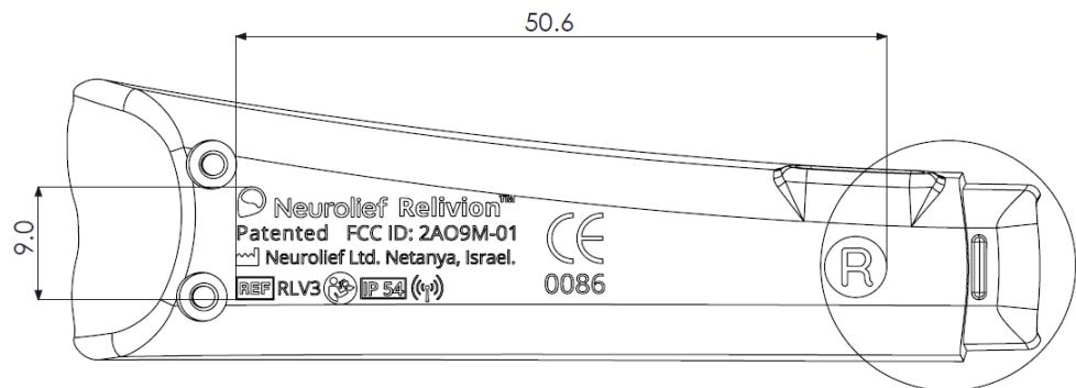
LABEL SAMPLE OF ETCHING ON DEVICE
