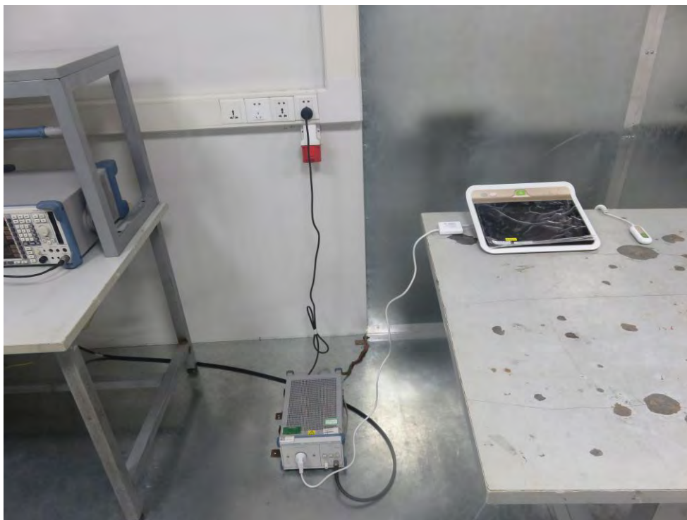
Photo of Conducted Emission Measurement
