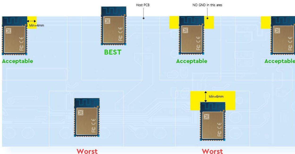
Figure 7: Recommended Module Mounting Examples
