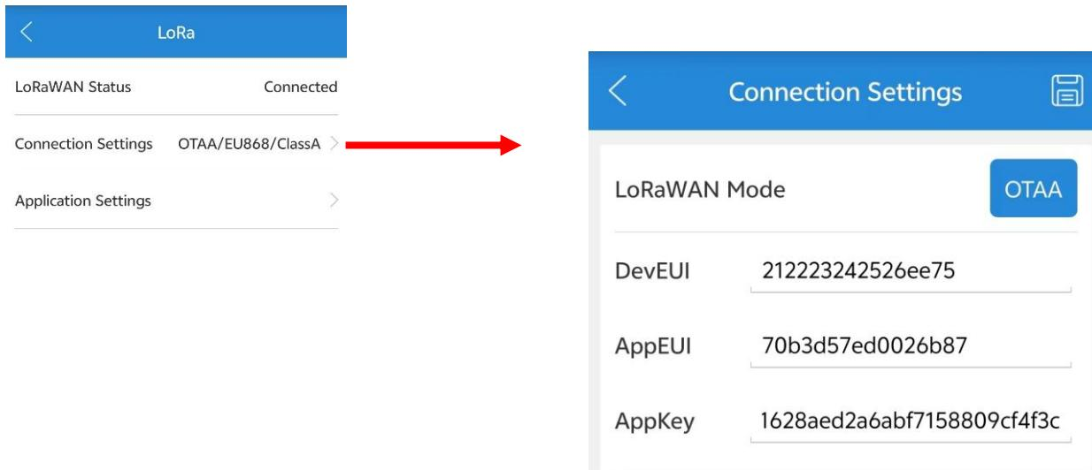
Configure/Read the LoRaWAN mode and the key parameters, such as DevEUI, AppEUI and AppKey.
