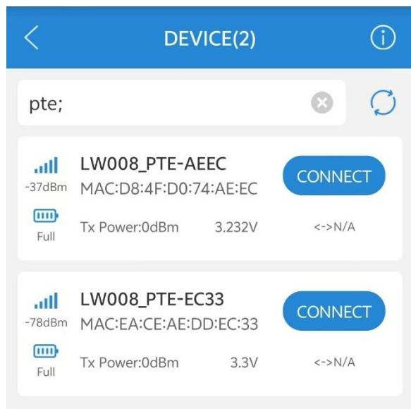
After the device is turned on, the device Bluetooth will start broadcasting. Open the MKLoRa APP and choose LW008, then you can search the LW008-PTE device by click the refresh icon. The default broadcast name of the device: LW008-PTE -XXXX. Then click “Connect” button, the default login password is Moko4321. The Edit Filter at the top can help user filter the keywords and RSSI. RSSI ranges from -127dBm to 0dBm;
