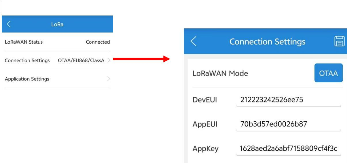
Configure/Read the LoRaWAN mode and the key parameters, such as DevEUI, AppEUI and AppKey.
