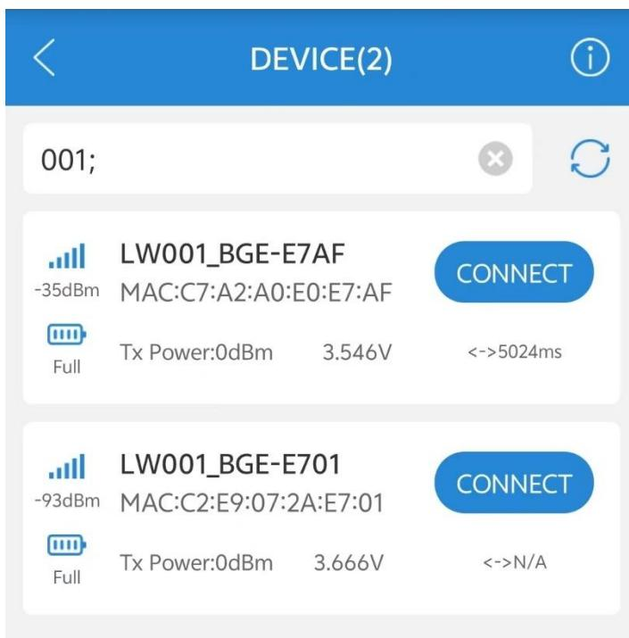
After the device is turned on, the device Bluetooth will start broadcasting. Open the MKLoRa APP and choose LW001, then you can search the LW001-BGE device by click the refresh icon. The default broadcast name of the device: LW001-BGE -XXXX.
