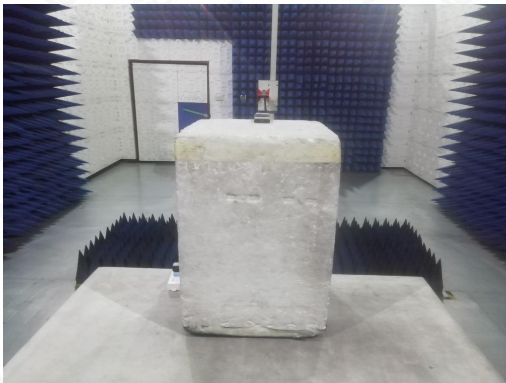
FCC RADIATED EMISSION TEST SETUP ABOVE 1GHZ
