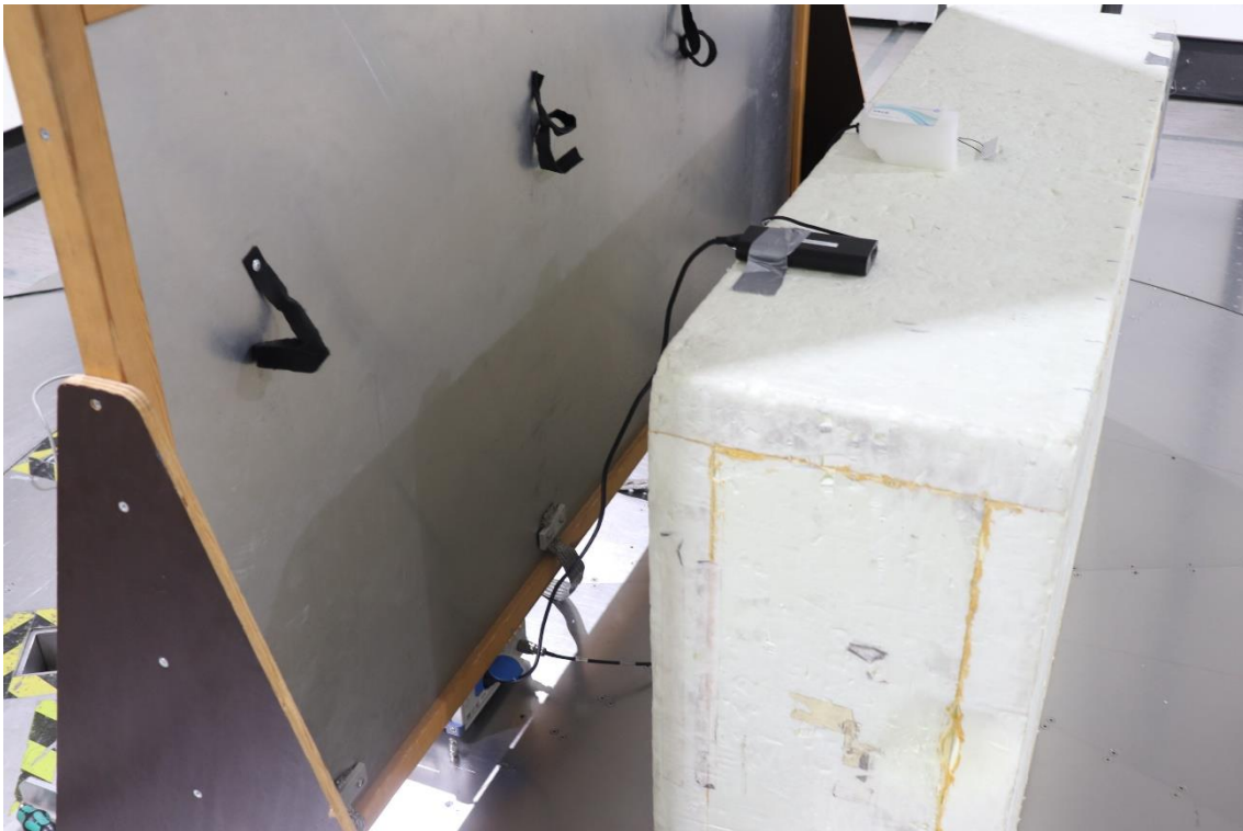
Photograph 1: Test setup for AC Power-Line Conducted Emissions
