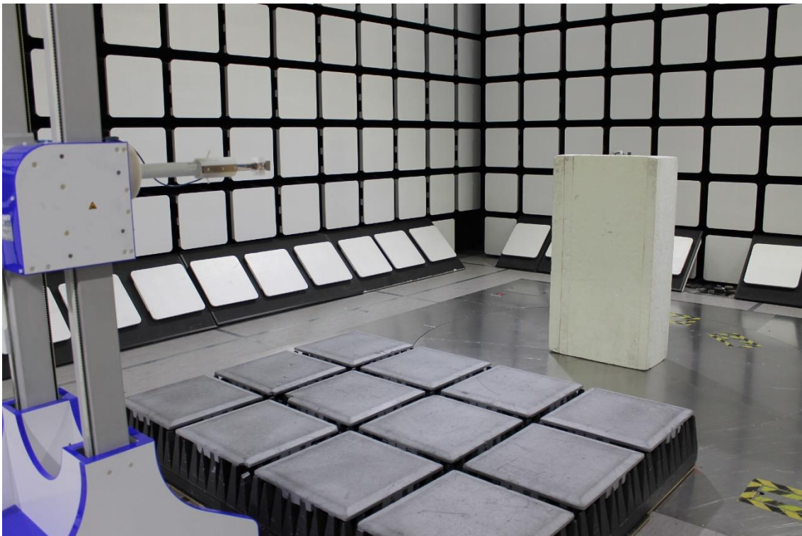
Photograph 4: Test setup for radiated emissions 18 – 26.5 GHz
