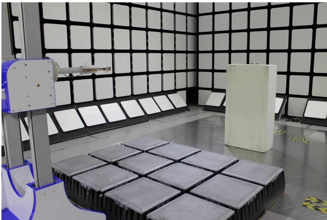
Photograph 5: Test setup for radiated emissions 18 – 26.5 GHz
