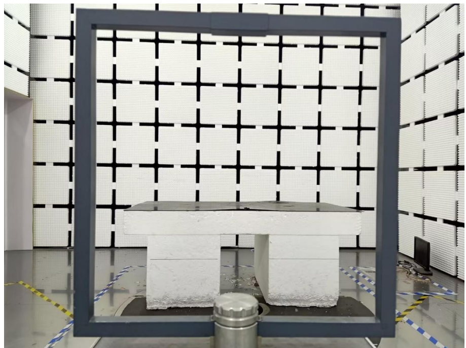
Radiation Emission Test Setup (Below 30MHz)
