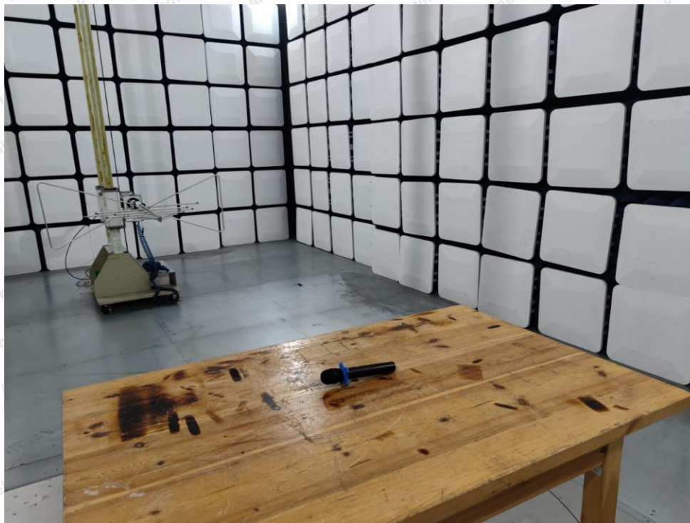
Photo of Radiation Emission Test
