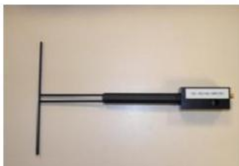
Figure 1 – Satimo COMOSAR Validation Dipole
