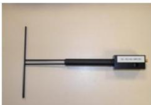
Figure 1 – Satimo COMOSAR Validation Dipole
