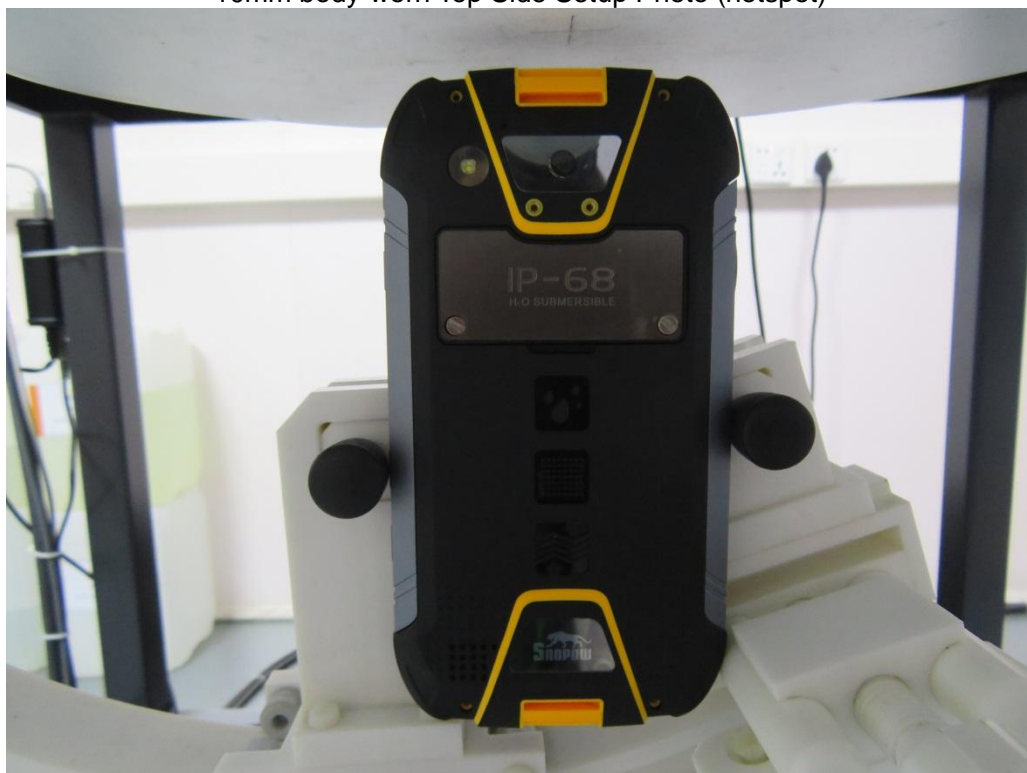
10mm body-worn Top Side Setup Photo (hotspot)
