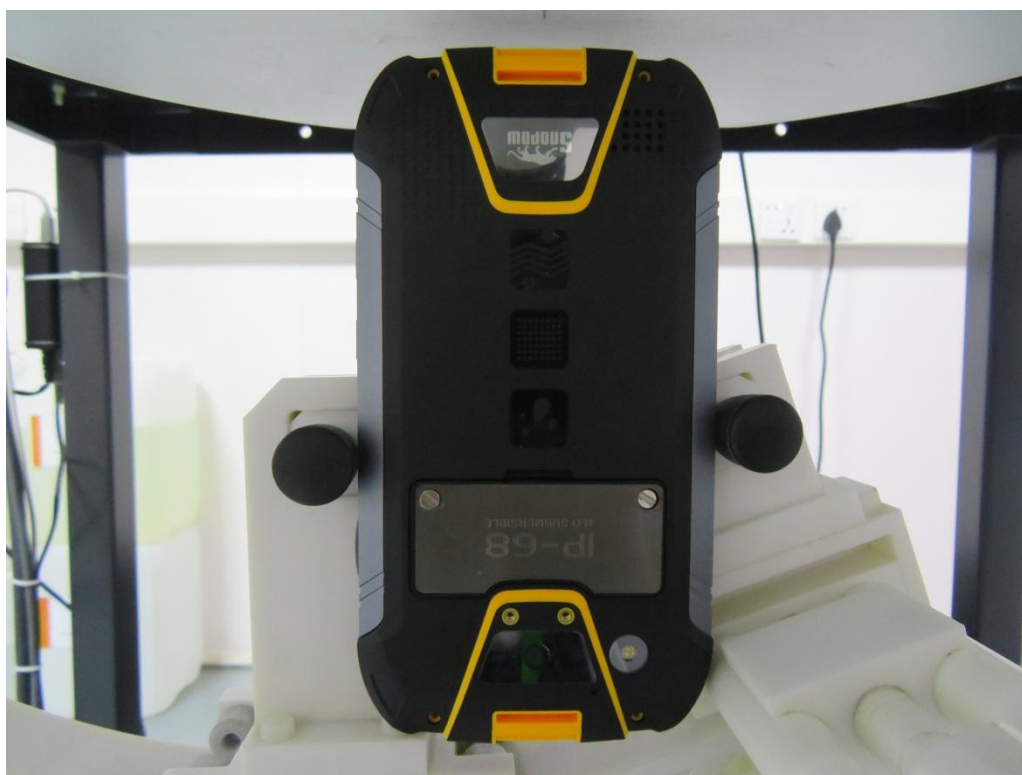
10mm body-worn Bottom Side Setup Photo (hotspot)
