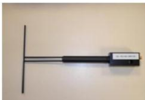
Figure 1 – Satimo COMOSAR Validation Dipole
