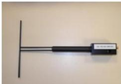
Figure 1 – Satimo COMOSAR Validation Dipole
