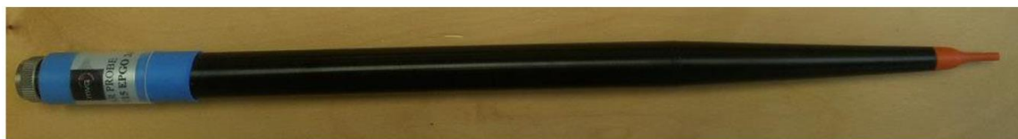
Figure 1 – MVG COMOSAR Dosimetric E field Dipole
