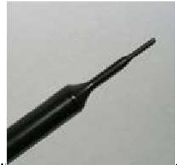
Figure 4.4 EX3DV4 E-field probe
