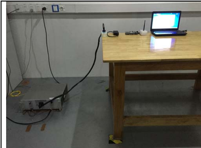
Conducted Emissions Test Setup Front View
