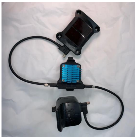
Figure 5: Silver Glade unit paired with both PV and TEG energy harvesting modules
