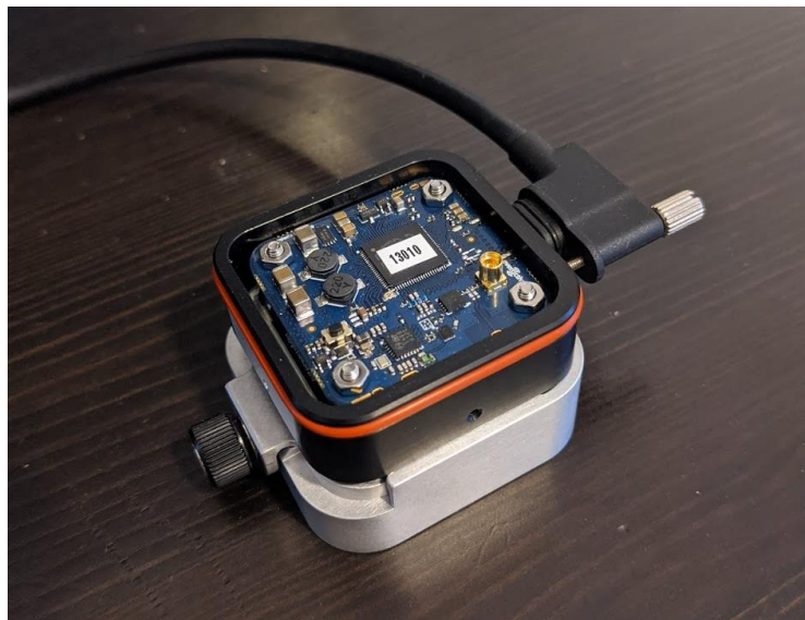
Figure 3: Silver Glade with cap and antenna removed for conducted wireless testing
