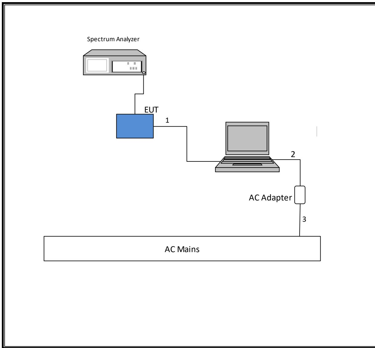
**SETUP DIAGRAM FOR RADIATED TESTS**
