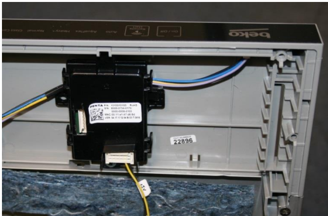
Location of transmitting antenna/module. Antenna separation distance to the surface tested is 12mm. Separation distance to other edges >25 mm.
