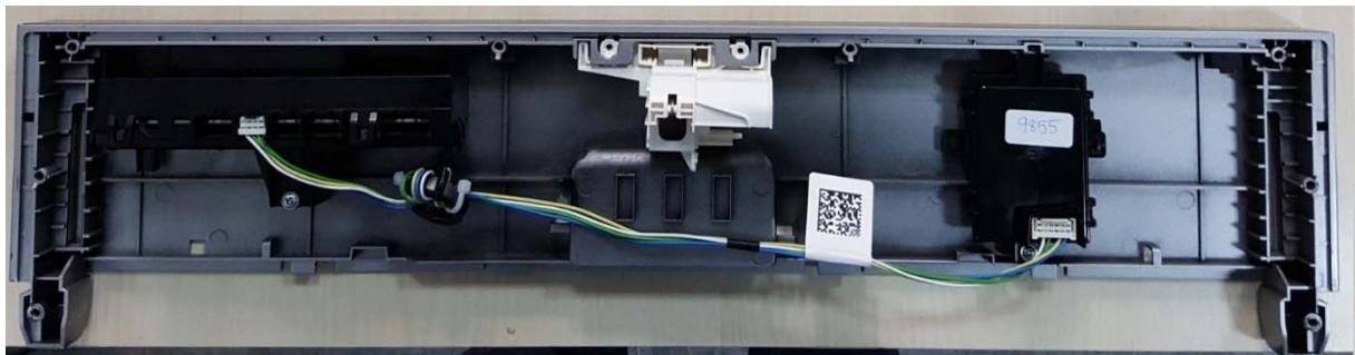
WeMod board is connected to display board via 4-pinned socket.
