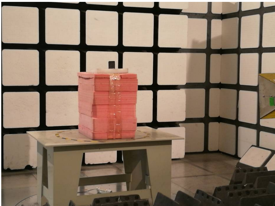
Radiated Emissions View (Above 1 GHz)
