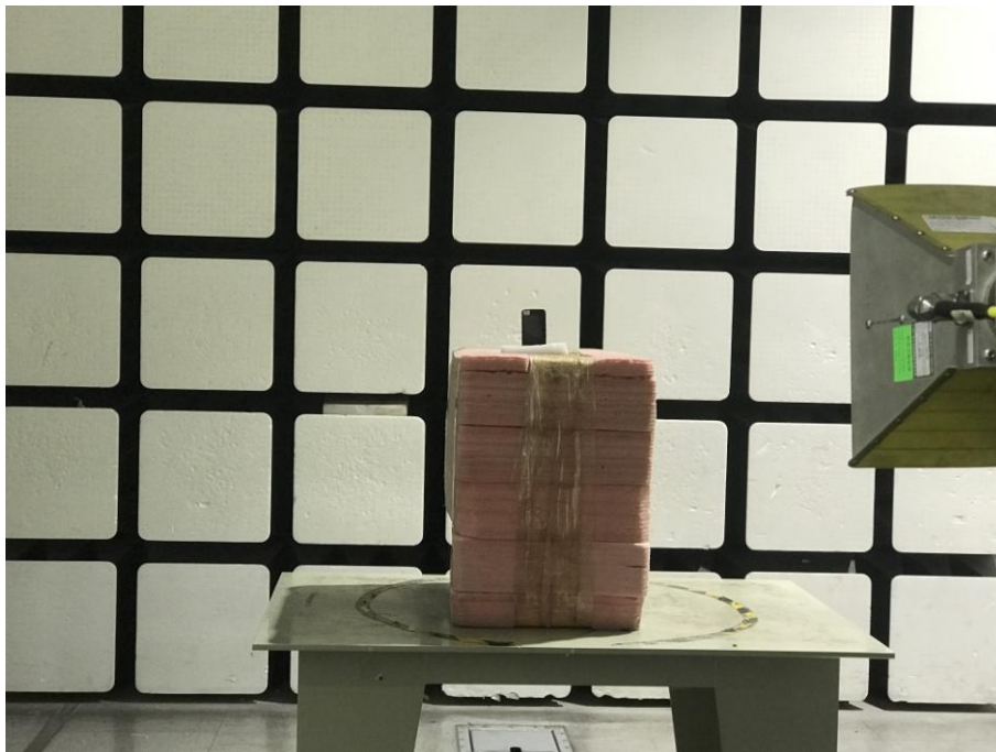
Radiated Emissions View (Above 1 GHz)
