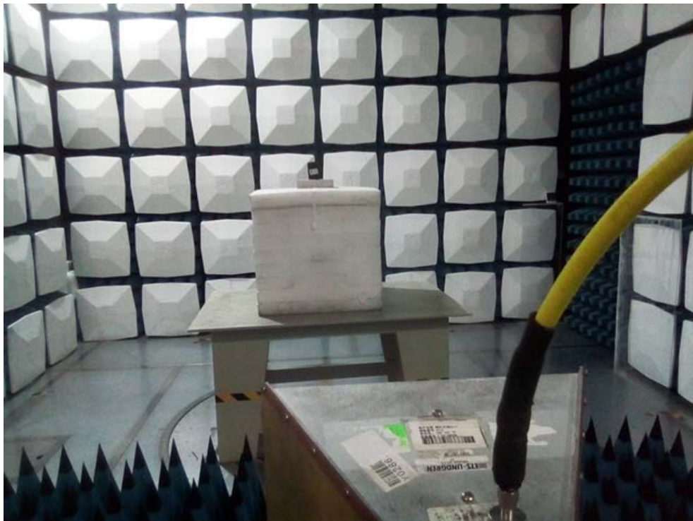
Radiated Emission Above 1GHz View
