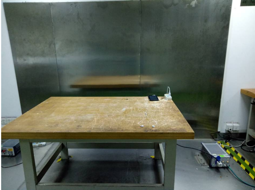
Conducted Emissions - Front View
