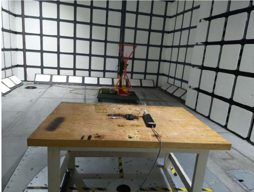
Radiated Emissions View (Below 1 GHz)
