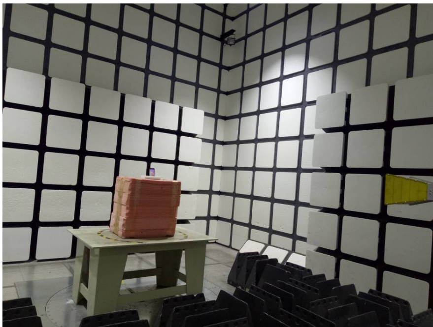
Radiated Emissions View (Above 1 GHz)
