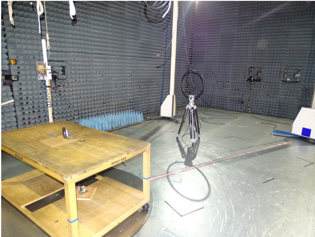
Photo 3: Test setup for radiated measurements (below 30 MHz)
