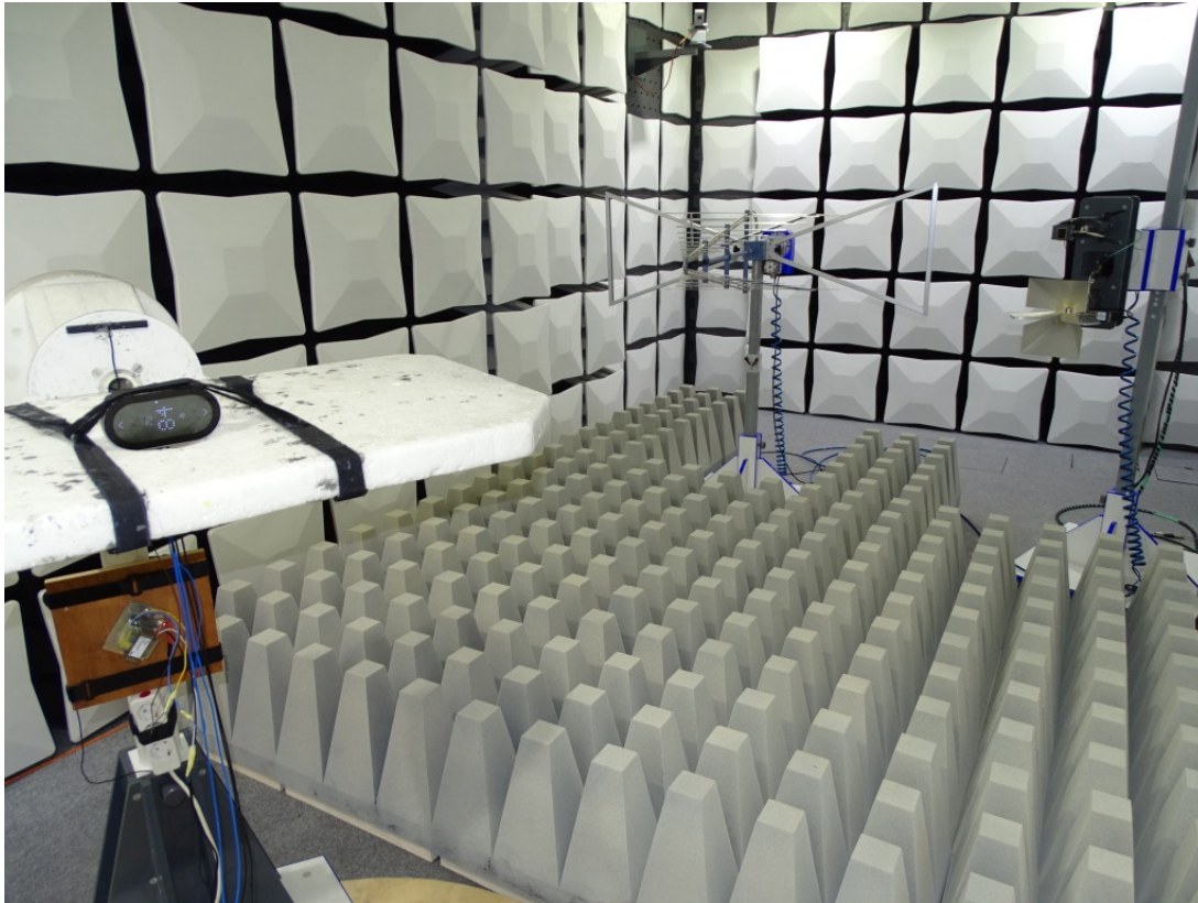
Photo 5: Test setup for radiated measurements (1 GHz to 26 GHz)
