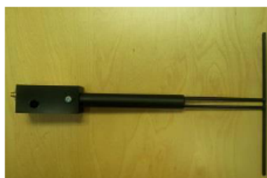
Figure 1 – MVG COMOSAR Validation Dipole
