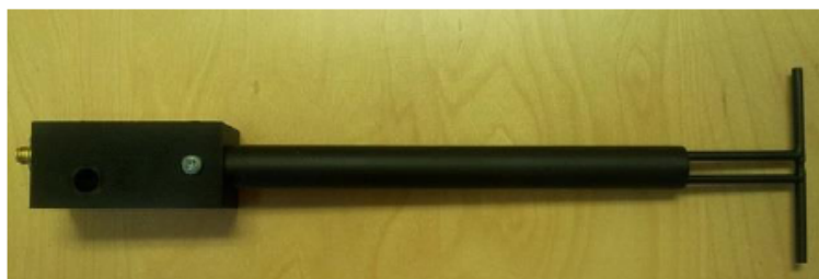
Figure 1 – MVG COMOSAR Validation Dipole
