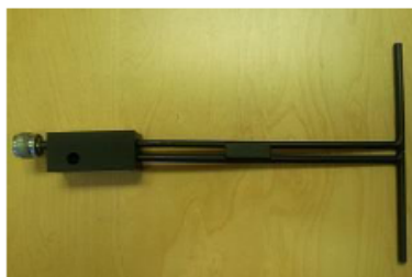
Figure 1 – MVG COMOSAR Validation Dipole
