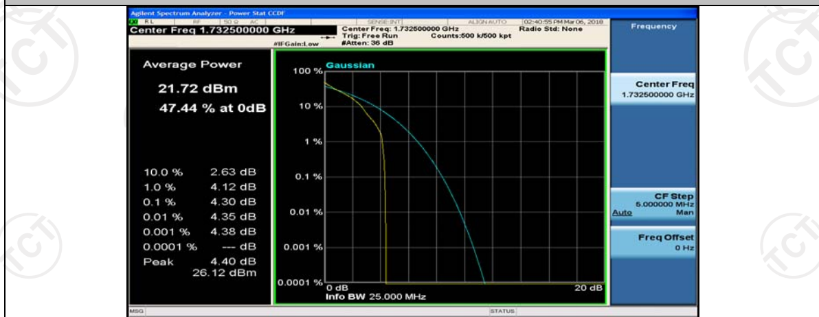
Channel Bandwidth: 10 MHz_MCH_QPSK_1RB#24
