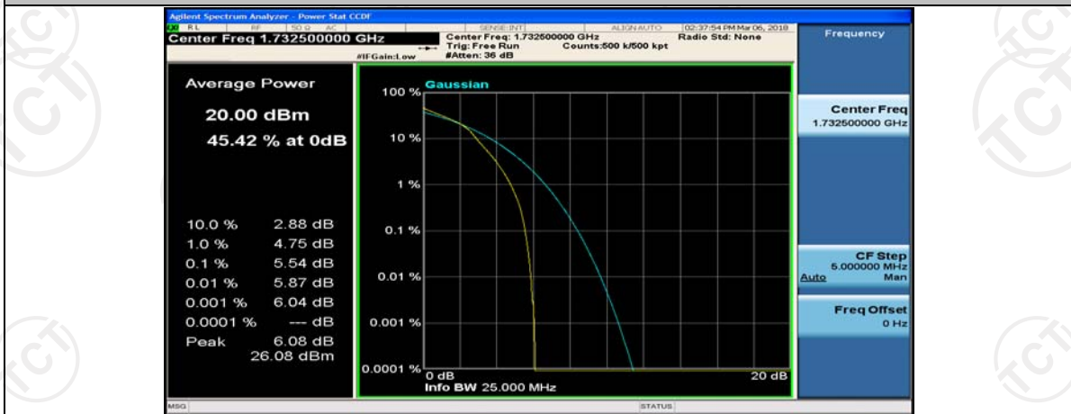
(Channel Bandwidth: 5 MHz)_MCH_16QAM_25RB#0
