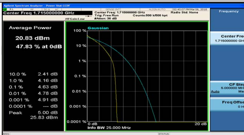
Channel Bandwidth: 10 MHz_LCH_QPSK_25RB#25
