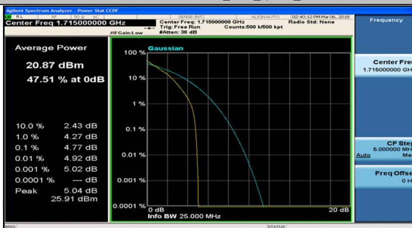
Channel Bandwidth: 10 MHz_LCH_QPSK_50RB#0
