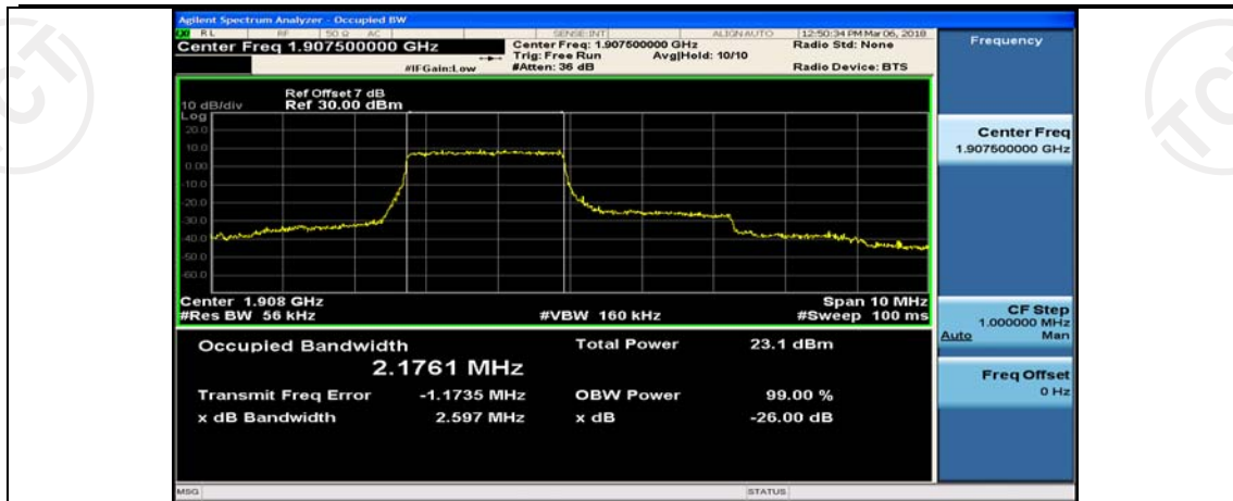
(Channel Bandwidth: 5 MHz)_HCH_QPSK_12RB#6
