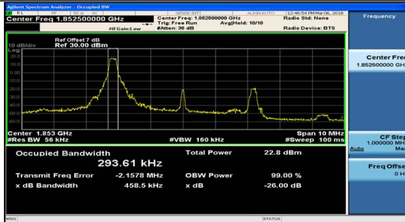
(Channel Bandwidth: 5 MHz)_LCH_QPSK_1RB#12
