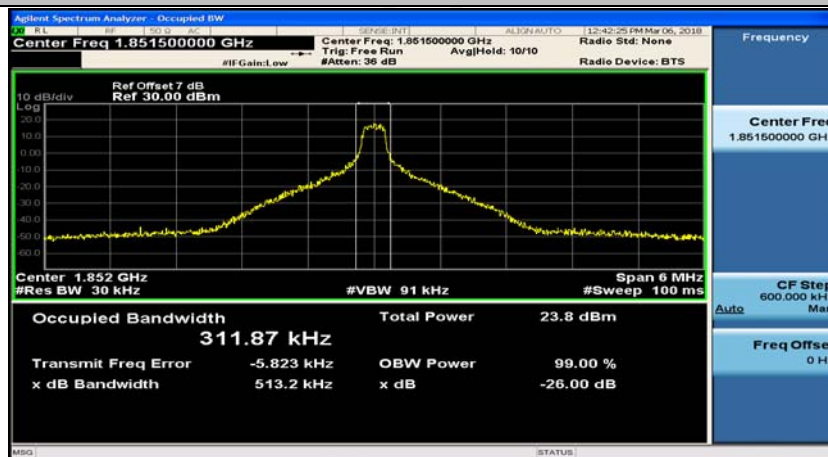
(Channel Bandwidth: 3 MHz)_LCH_QPSK_1RB#14
