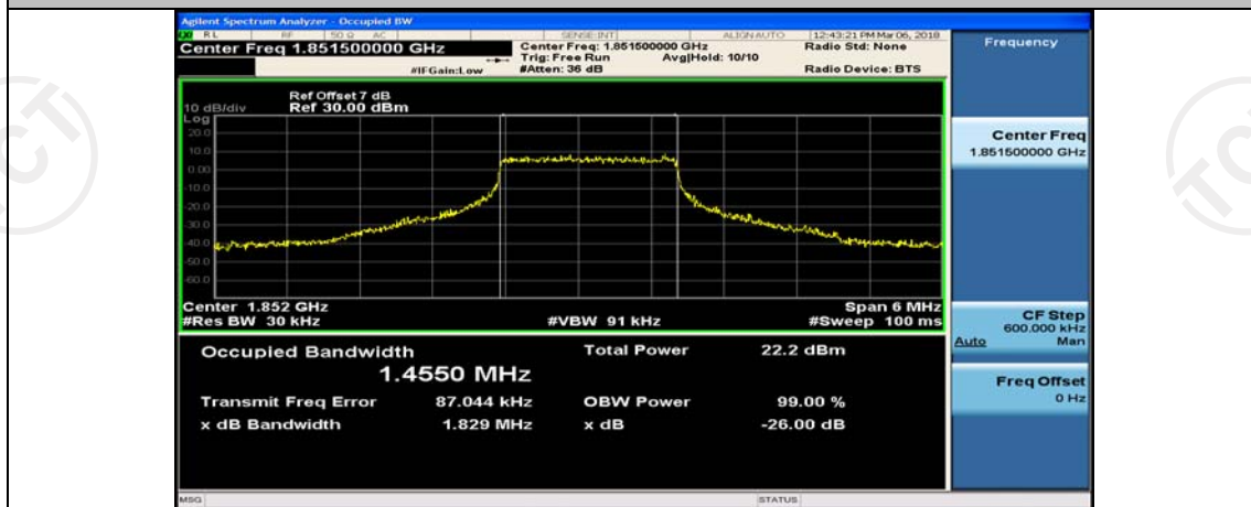
(Channel Bandwidth: 3 MHz)_LCH_16QAM_8RB#7
