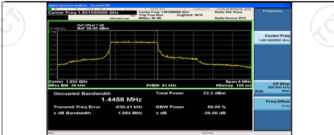
(Channel Bandwidth: 3 MHz)_LCH_16QAM_8RB#4
