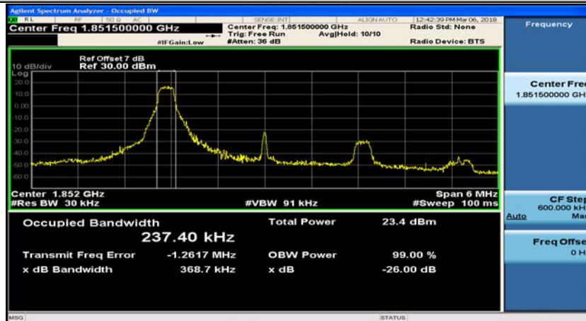
(Channel Bandwidth: 3 MHz)_LCH_16QAM_1RB#7
