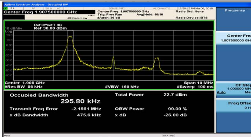
(Channel Bandwidth: 5 MHz)_HCH_16QAM_1RB#12
