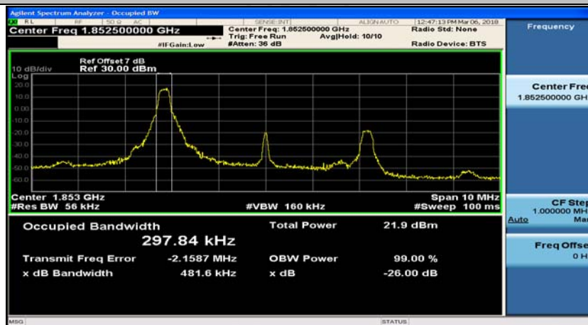
(Channel Bandwidth: 5 MHz)_LCH_16QAM_1RB#12
