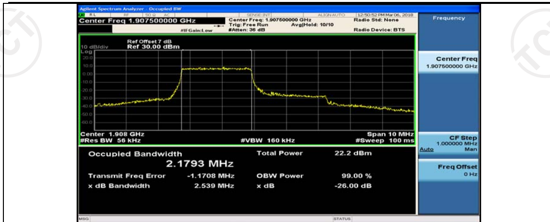
(Channel Bandwidth: 5 MHz)_HCH_16QAM_12RB#6
