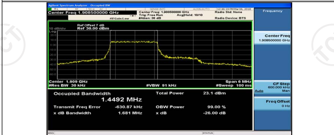
(Channel Bandwidth: 3 MHz)_HCH_16QAM_8RB#4
