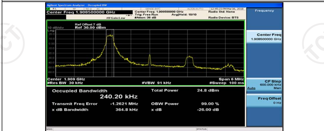
(Channel Bandwidth: 3 MHz)_HCH_QPSK_1RB#7
