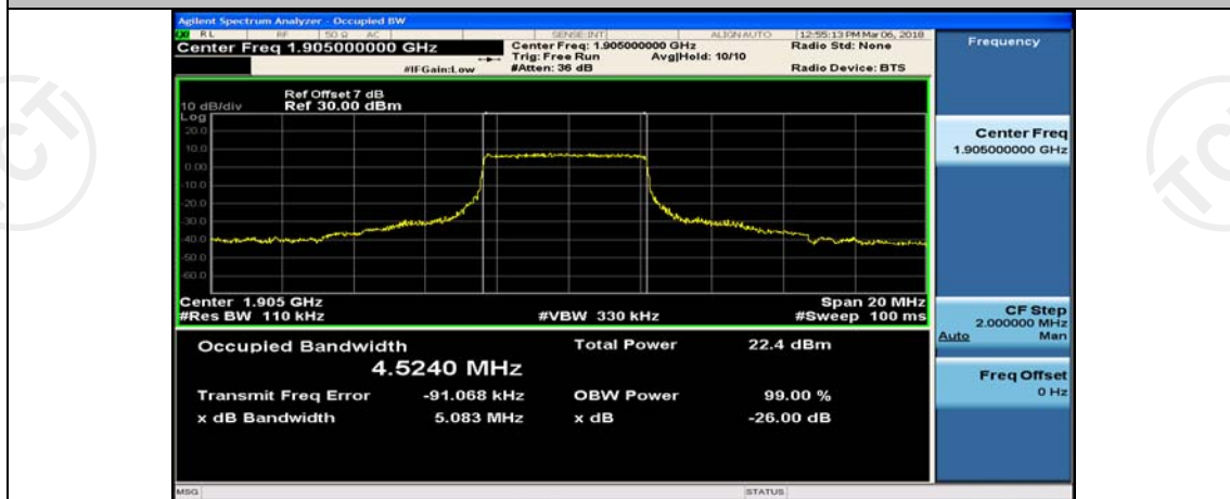
Channel Bandwidth: 10 MHz_HCH_QPSK_25RB#25
