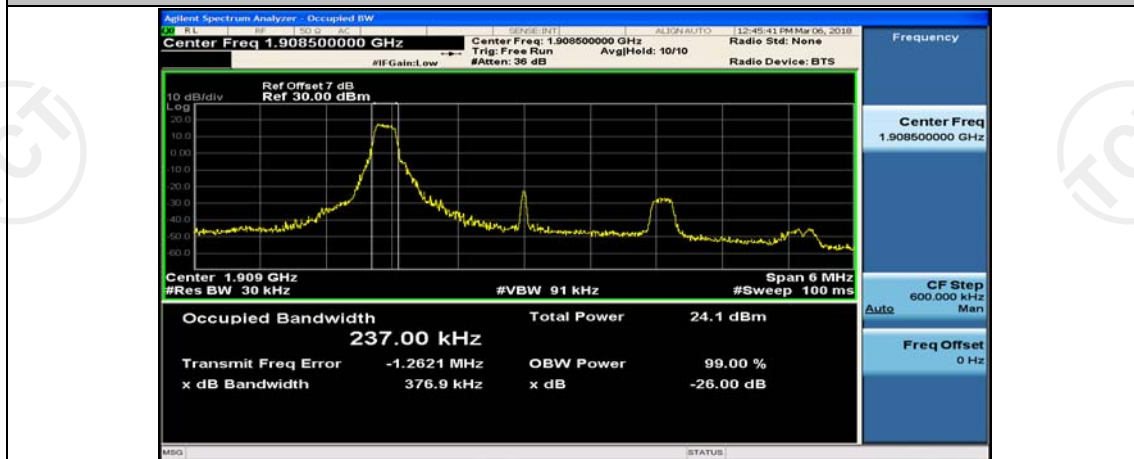
(Channel Bandwidth: 3 MHz)_HCH_16QAM_1RB#7
