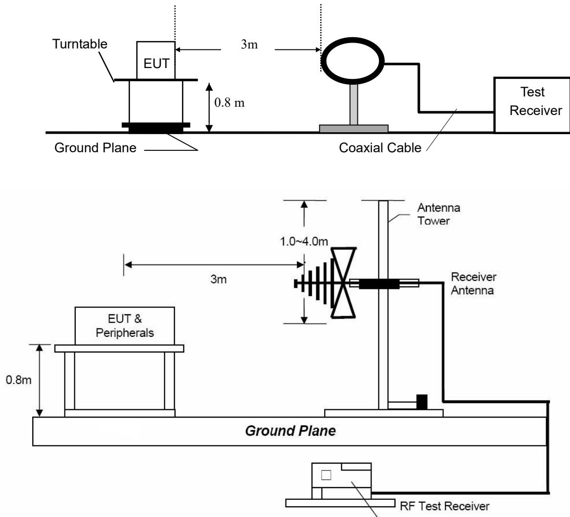
(2) Radiated Emission Test Set-Up, Frequency above 1GHz
