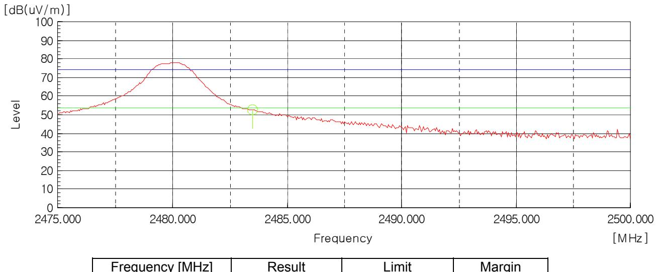
AV Detector: RBW: 1 MHz, VBW: 10 Hz (2 483.5 MHz - 2 500 MHz), Worst case (High, Vertical)
