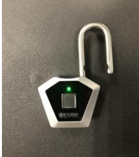
1.2 Put your fingers on the fingerprint collector, the indicator lights flicker and turn off, then lift your fingers and press the fingerprint collector again, the indicator lights flicker and turn off, repeat this process for three times. If registration is successful, the indicator light will be on for a whole second; if registration is failed, the light will flicker two times.
