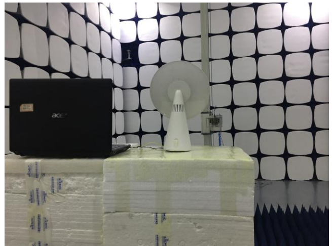
Radiated Spurious Emissions Test Setup Above 1GHz
